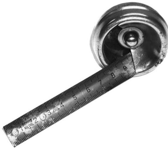
Fig. 1. Steel tape measure (ca. 1950). Note that the transverse curvature of the extended tape and the longitudinal curvature of the coiled tape are in the same sense.
